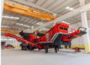
PRODUCTIVE IMPACT CRUSHER AND EFFICIENT VIBRATING SCREEN ON ROBUST CHASSIS AS SINGLE UNITE
